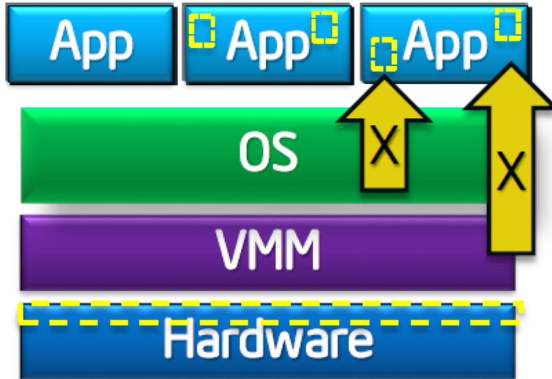
An enclave within an app is protected from interference from other software, including the OS and VMM. Note that enclaves can only run in ring 3 (user space).
